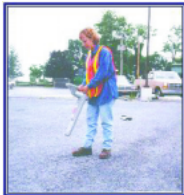
Figure 1 A radio frequency line locator mapping utilities
