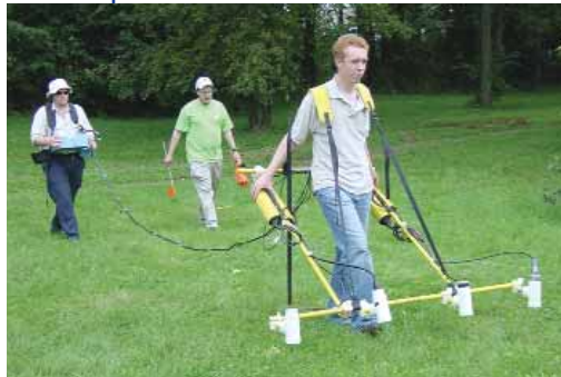
ARM and G-tek geophysicists conducting a magnetic survey with a G-tek TM-4.
