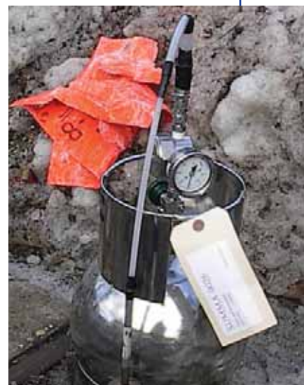
Summa canister for collection of air samples for VOC analysis
