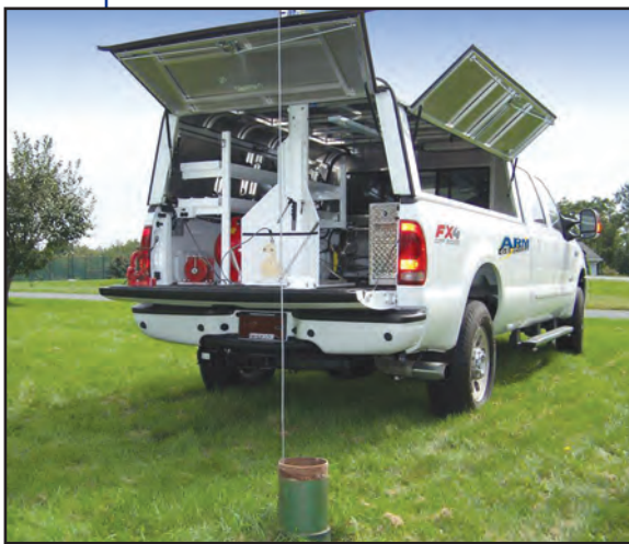
ARM's new geophysical logging truck
