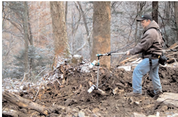
ARM geophysicist conducting magnetic survey
